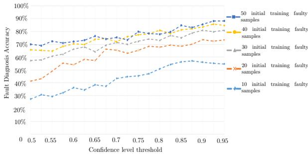
Figure 3: Experimental results showing the averaged diagnostic accuracy rates versus various confidence level thresholds.
