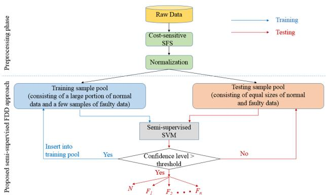
Figure 1: The flowchart of the proposed semi-supervised FDD approach for AHU faults.
